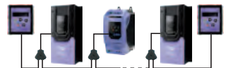
Two Optipoint 2 with multiple Optidrives (up to 63 max)
